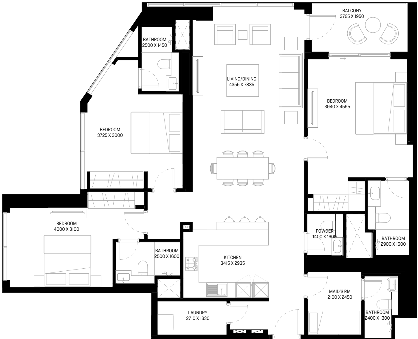
TYPICAL FLOOR PLAN (10,14,16,22,26,28,32)_LOWER LEVEL
